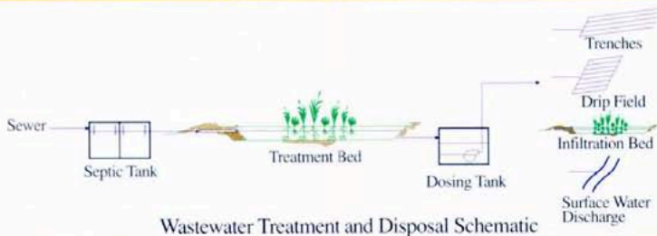
Wastewater Treatment and Disposal Schematic
